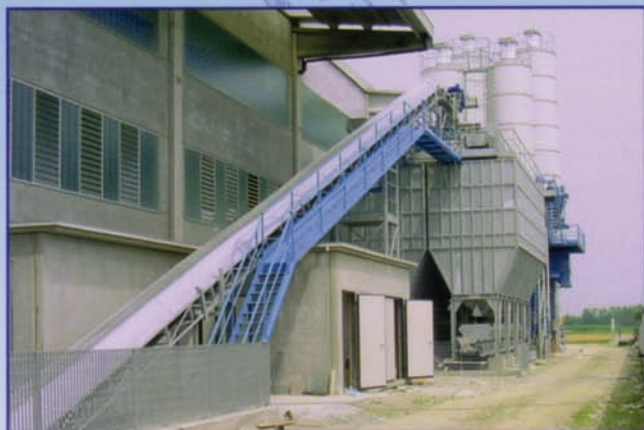
Receiving hopper and belt conveyor with anti-dust galvanised cover.
